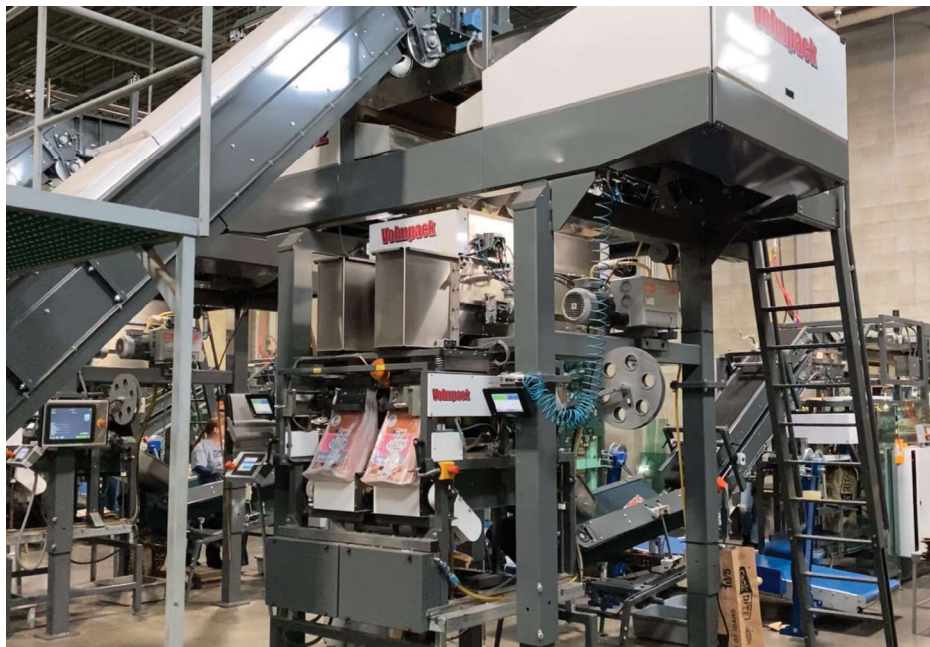
Volm Companies was instrumental in introducing automated weighing equipment such as the Volmpack weigher and wicket bagger to the North American marketplace.
