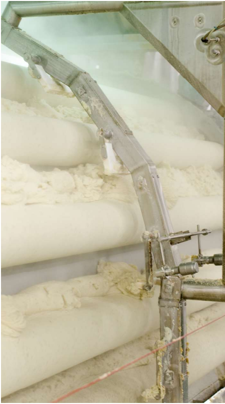
Above: Just one step in the potato flake and flour manufacturing process involves product going through rollers of the drying drum.
