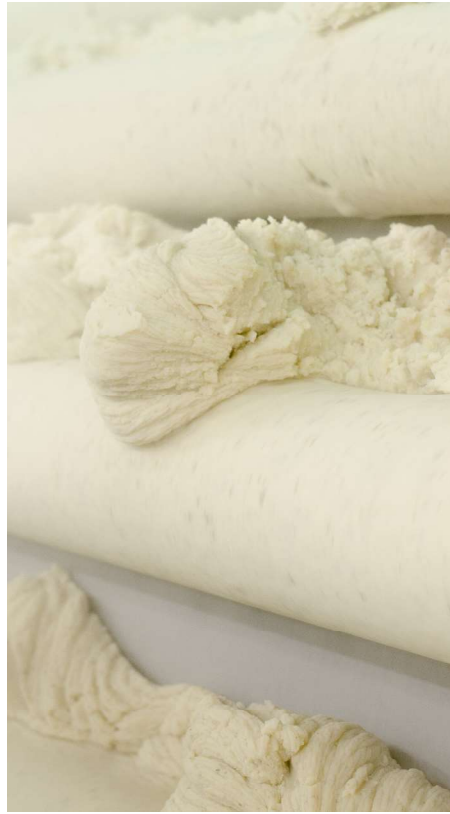
Above: Just one step in the potato flake and flour manufacturing process involves product going through rollers of the drying drum.
