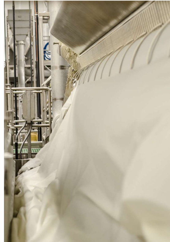
Above: Once through the exit side of the drum shown here, the product is essentially potato paper.
