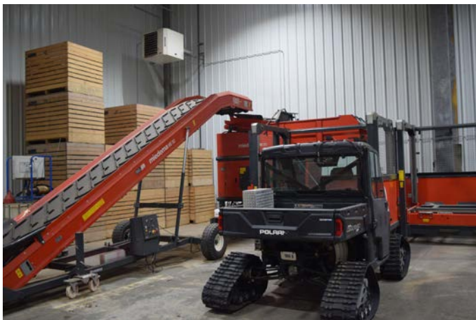
An automatic boxer, the Miedema ME 80 with wide, troughed conveyor belt, was purchased from T.I.P., Inc., of Custer, Wisconsin.
