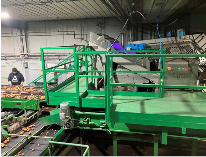
As part of a fabrication project for Midwestern Potatoes, Chris Anderson built the catwalk around the operation's grading and sorting line.
