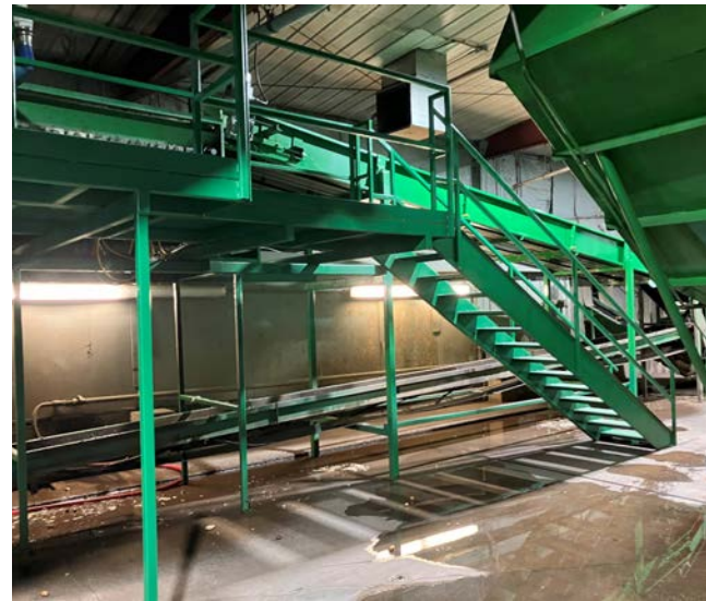
As part of a fabrication project for Midwestern Potatoes, Chris Anderson built the catwalk around the operation's grading and sorting line.
