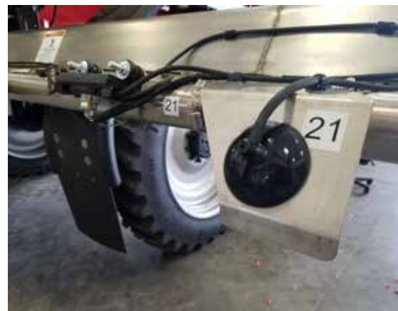
A precision ag specialist for Heartland AG Systems, Ryan Culver installs an Intelligent AG dry fertilizer blockage monitor on a new 72-foot Salford RA-855 Air Boom Spreader.
