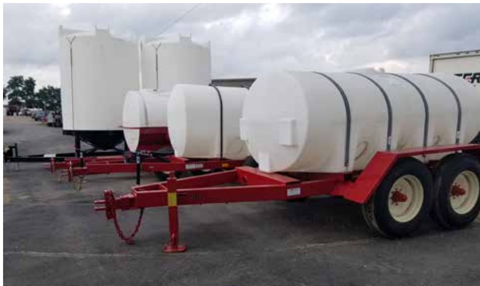
Heartland AG Systems in DeForest, Wisconsin, offers nurse trailers that hold 1,000-2,000 gallons and storage trailers that carry 6,000 to 9,000 gallons. All trailers are plumbed up to the customer’s specifications.
