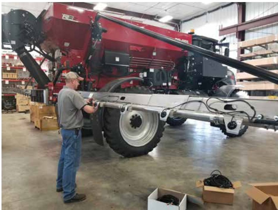
A precision ag specialist for Heartland AG Systems, Ryan Culver installs an Intelligent AG dry fertilizer blockage monitor on a new 72-foot Salford RA-855 Air Boom Spreader.
