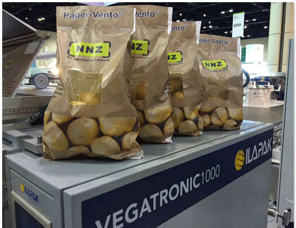
Marty Kolpack assures that the Paper Vento bags with mesh windows run excellently on the ILAPAK VFFS (Vertical Form-Fill Seal) Vegatronic 1000 baggers.
