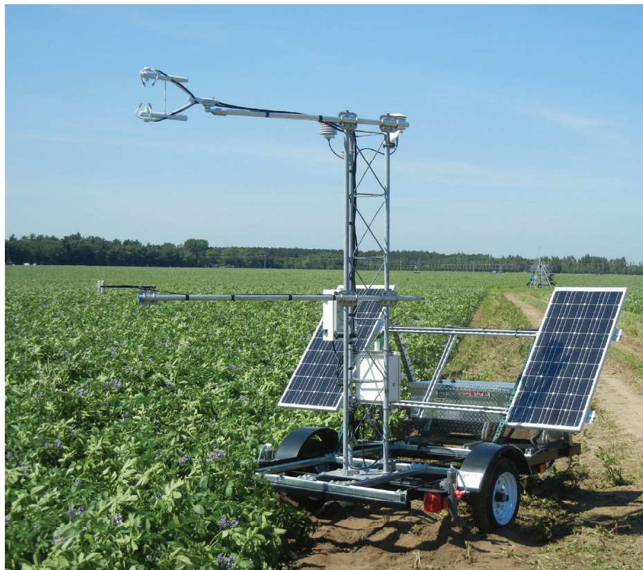
Eddy covariance flux towers are being used in Central Wisconsin to accurately measure evapotranspiration (ET), which helps growers with their irrigation management.
