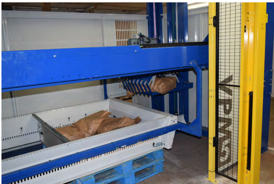
A Verbruggen VPM-5 automatic palletizer is hard at work stacking bales of potatoes at Potato Plant, Inc.
