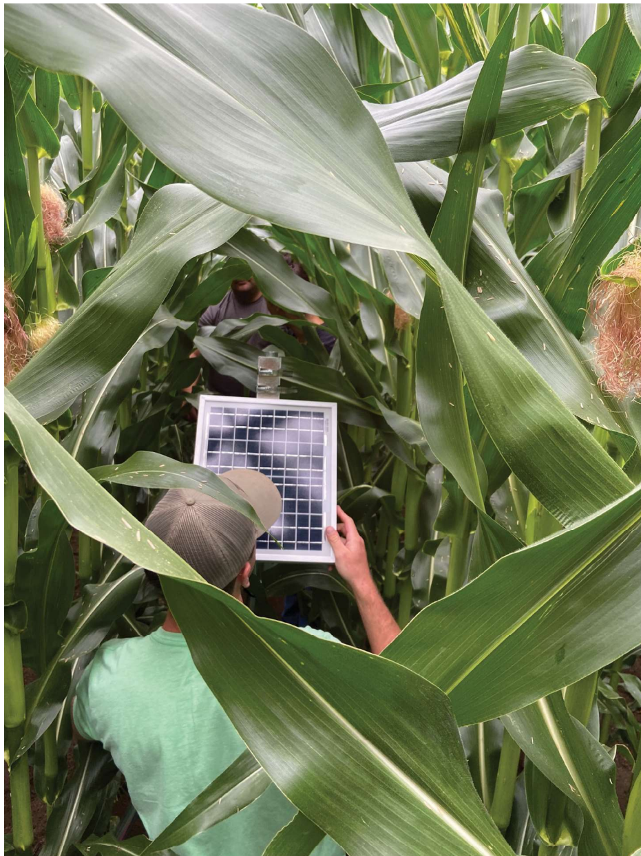
The solar-powered probes have sensors that record soil moisture and temperature at six depths down to 40 inches, and then transmit data that is accessible in real time to the farmers. Two probes were placed in each of the 30 fields across Wisconsin and Minnesota.
