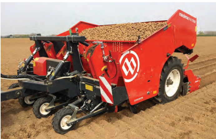
T.I.P., Inc. just sold a Miedema CP42 four-row cup planter to a seed grower in Antigo, Wisconsin. It combines seedbed preparation, planting, and ridging capabilities in a single pass, and features a large bunker and potato-friendly planting elements.
