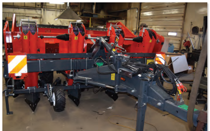
T.I.P., Inc. just sold a Miedema CP42 four-row cup planter to a seed grower in Antigo, Wisconsin. It combines seedbed preparation, planting, and ridging capabilities in a single pass, and features a large bunker and potato-friendly planting elements.
