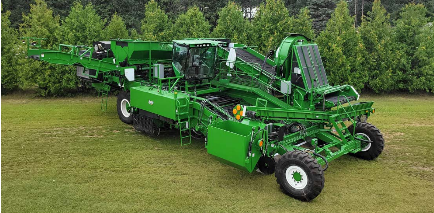
The photo taken at Schroeder Bros. Farms, Antigo, Wisconsin, is of an Advanced Farm Equipment 2022 4-Row Self-Propelled Potato Harvester with a 65-inch AirHead.
