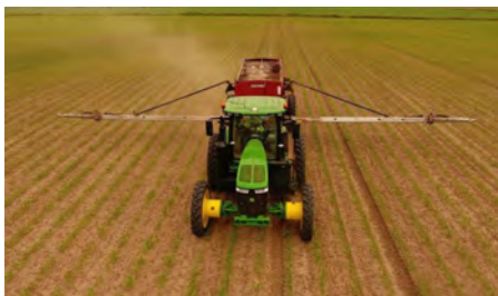
Hooked up to a John Deere 7210R, a Salford AirFlow with 60-foot booms is used to spread fertilizer in sweet corn, July 2021. Image courtesy of John Schomburg, Roven Farms Photography
