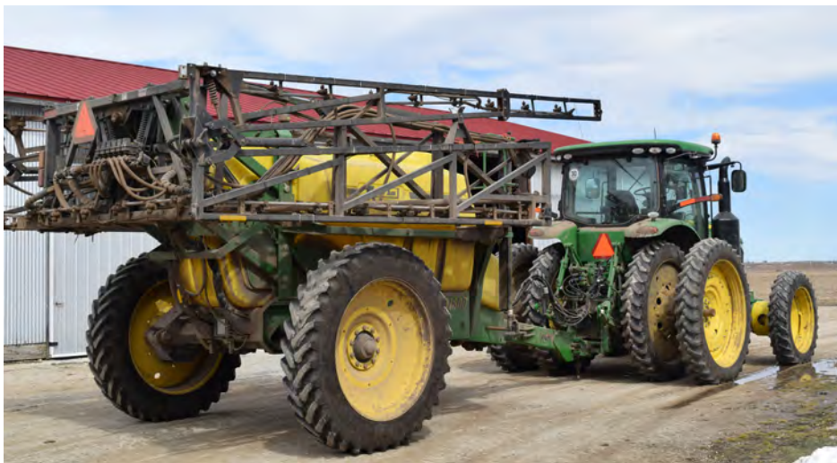
The sprayer owned by Allan Brooks features RTK guidance, auto steer, 54 nozzles, and six 16-foot sections for 90 feet of boom.
