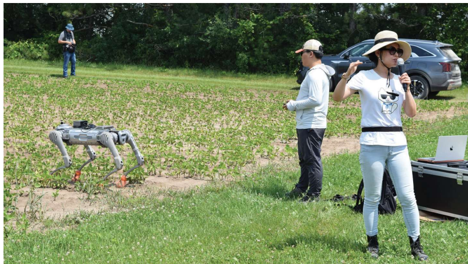
HARS Field Day attendees enjoyed seeing a 100-pound robot that Yi Wang (right) and her team acquired this year and is the perfect size for scouting snap bean and green pea fields. She outfitted the droid with orange Crocs™ so its lower appendages won’t damage the soil. Even wearing Crocs, it hops and turns.
