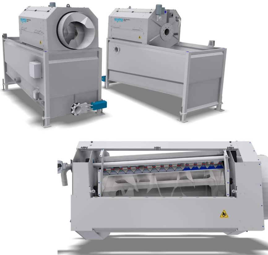
Above: The Wyma Solutions Rotary Drum Filtration System is used to remove organic matter and other debris from a water stream for water reuse or before finer filtration by the Micron Filter. The Rotary Filter reduces freshwater consumption in vegetable washing, food processing and industrial use by up to 95%, depending on the application.
