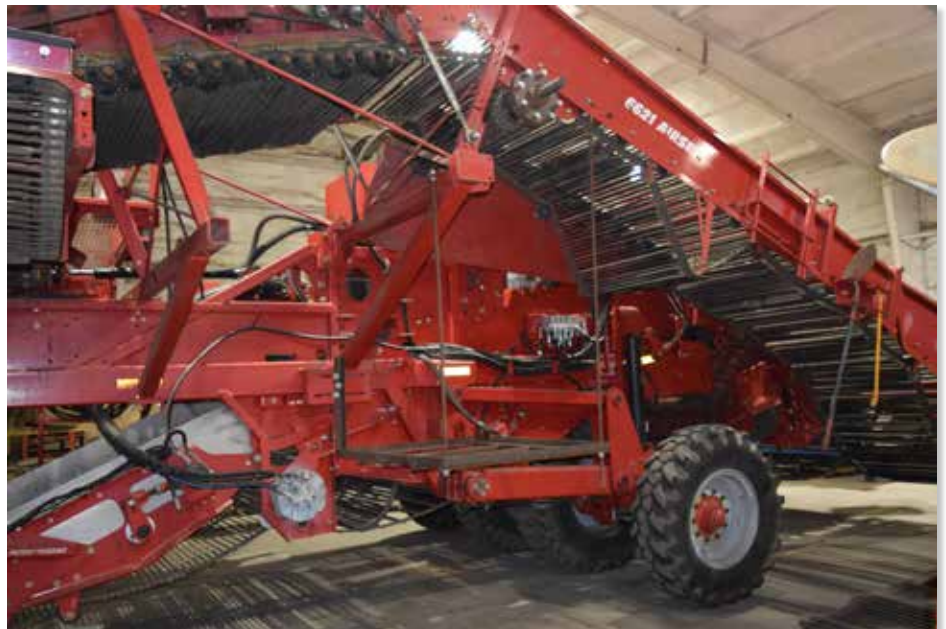
Above: Links on the chain of the Spudnik 6621 AirSep potato harvester are close together for digging Creamer potatoes for The Little Potato Company.
