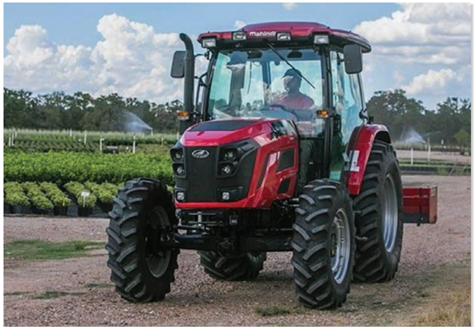
The Mahindra Model 8090 utility tractor with a 4-cylinder turbocharged, intercooled diesel engine and air-conditioned cab is mainly used for agricultural applications.
