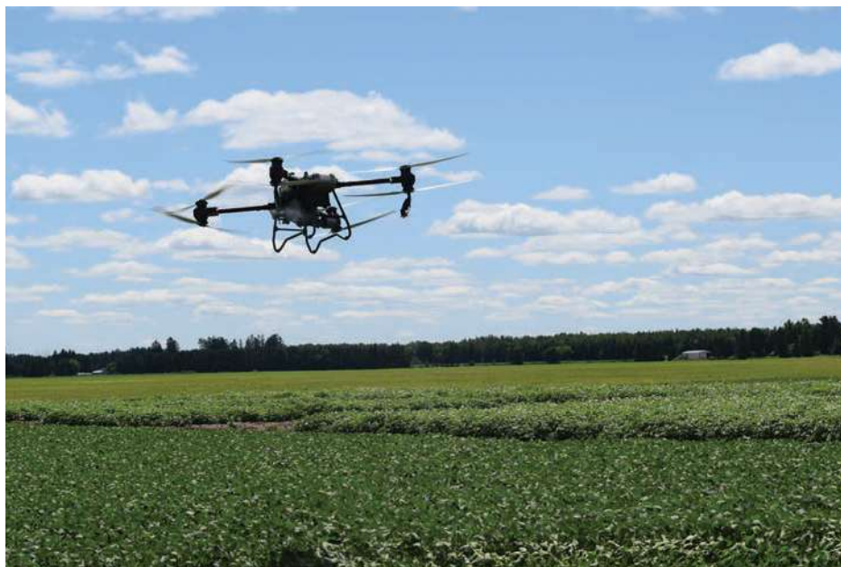
During the LARS Field Day on July 17, Angel Zarda and Scott Houdak of Venture Ag Drones gave a spraying demonstration over a soybean field using blue dye so those in attendance could inspect the plants afterwards to evaluate coverage.
