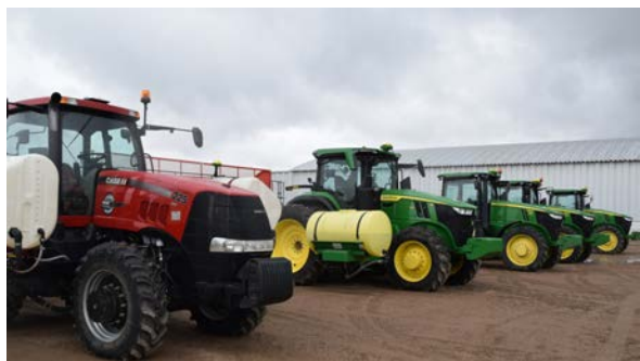
Above & Below: Though Guenthner Potato Company is largely a John Deere operation, the first tractor in the lineup is a Case IH Magnum 225 CVT set up for tillage, while second in line stands a John Deere 7R 310 hooked up to a Harriston cup planter.
