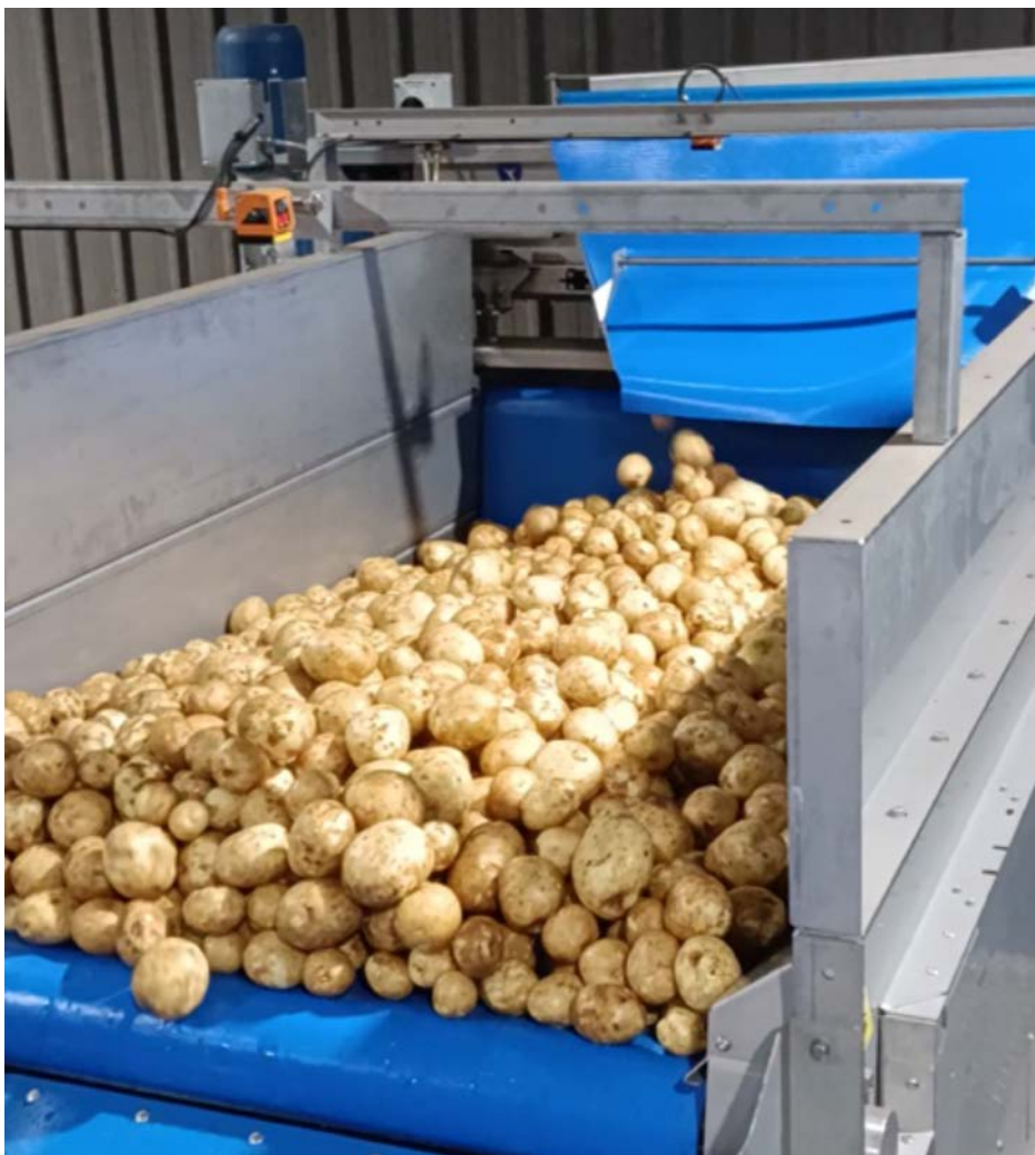
Left: Evenflow hoppers ensure continuous and controlled feed of potato and vegetable crops into a handling line, whether grading potatoes, washing carrots or packing onions.
