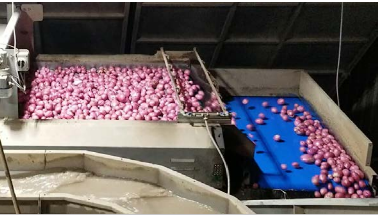
Above and Right: Absorbent Flat Bed Dryers and Drying Rollers remove surface moisture from potatoes before inspection or packing.
