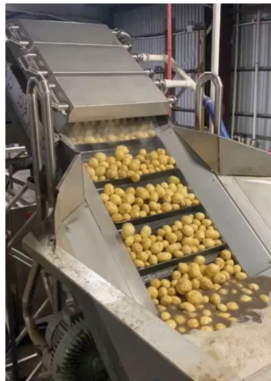
Above: Wyma Solutions Wet Hoppers are used in receiving, soaking, pre-cleaning, buffering and regulating potato flow into a packing plant.
