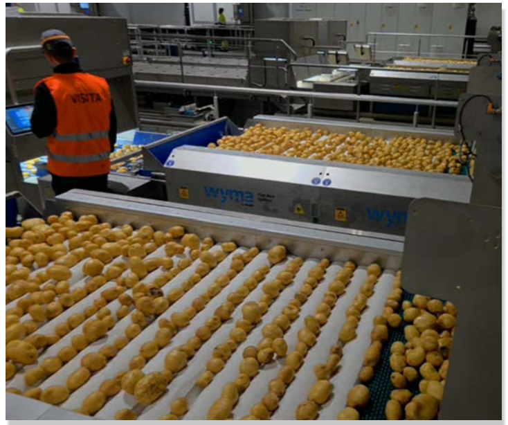
Above and Right: Absorbent Flat Bed Dryers and Drying Rollers remove surface moisture from potatoes before inspection or packing.
