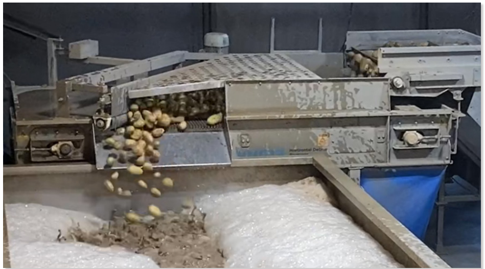
The Wyma Solutions Horizontal Debris Remover separates dirt, vines, and other field debris from potatoes.
